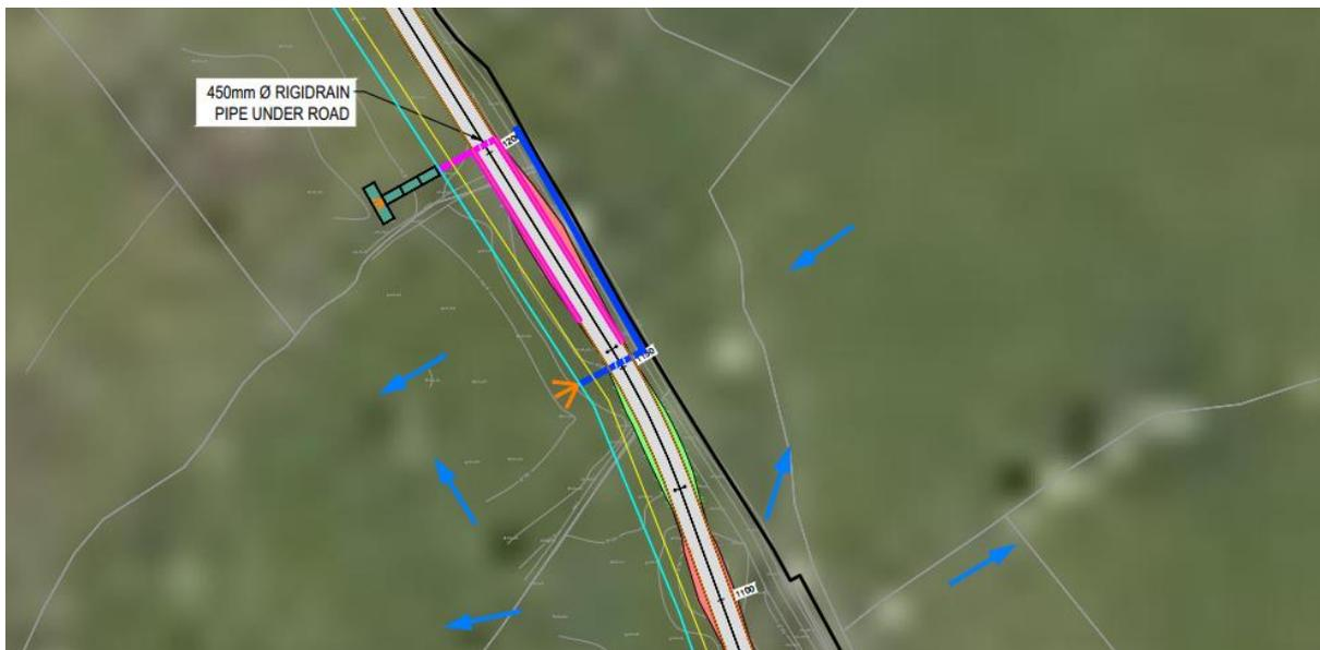
Figure 1 – Typical drainage design
