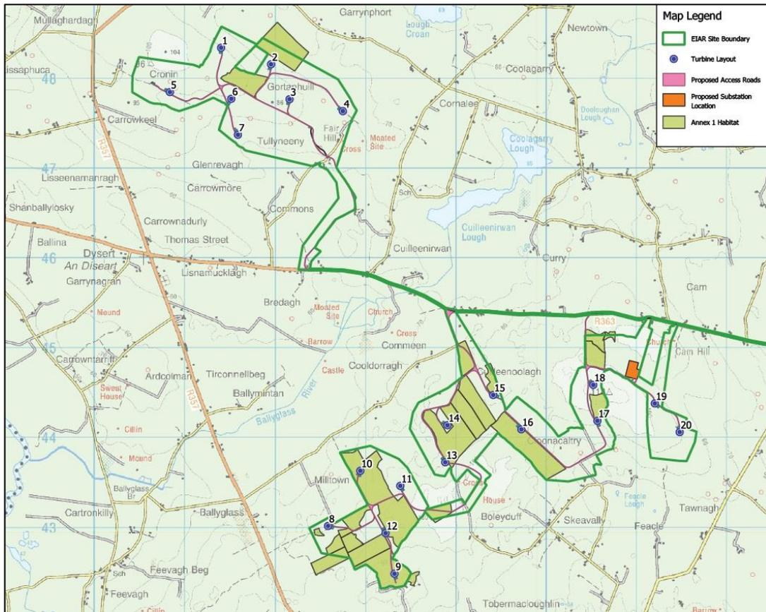
Figure 3-6 Fourth Site Layout (Revised 20 Turbine Layout Accounting for Annex I Habitat and Telecoms)
